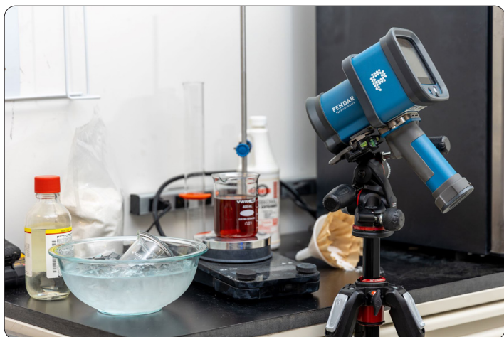
Pendar X10 identifies unknown substances in a clandestine lab.
